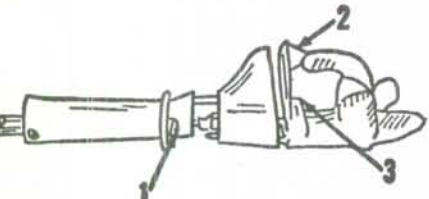
Fig. M1-15—Partially disassembled view of the three-piece lower unit showing location of the two stud nuts (1 & 3) and the retaining screw (2) which hold lower unit together. Refer to text for disassembly procedure.
