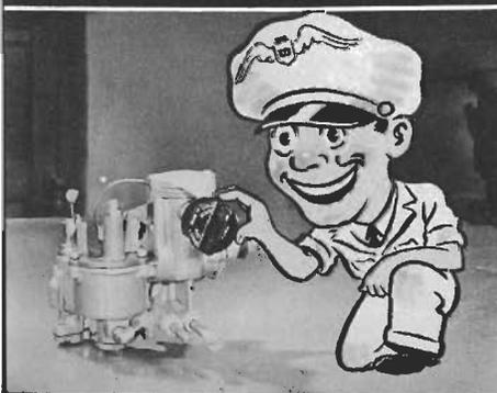
**PUTT:** But when the motor is cold and you want a richer mixture to get it started, you turn the dial to the "Cold Start" position.
