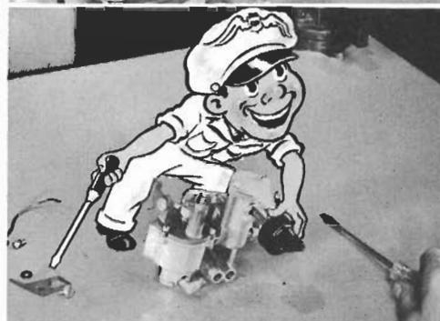
**PUTT:** Slip the angled end of the lever into the hole in the vent needle and the other end on the cam at the end of the choke shaft assembly.
