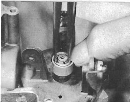
**PUTT:** The lock pin goes through the holes in both the dome and the needle. Bend the pin around the dome at both ends and it's in to stay. That's it.
