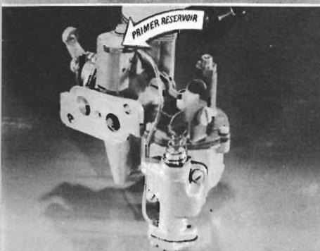
**PUTT:** And a primer reservoir up here. In between the primer body and the primer reservoir is . . .
