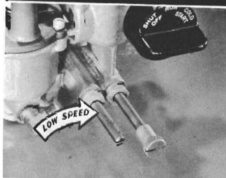
**PUTT:** A fuel line from here carries fuel up to the inlet hole in the low speed inlet port that opens into the crank case.
