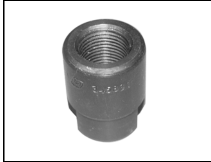
Remover, prop shaft / bearing housing 002628 P/N 345831 (40/50, 60/70, 90-140, 200/225) Use with P/N 391008 slide hammer
