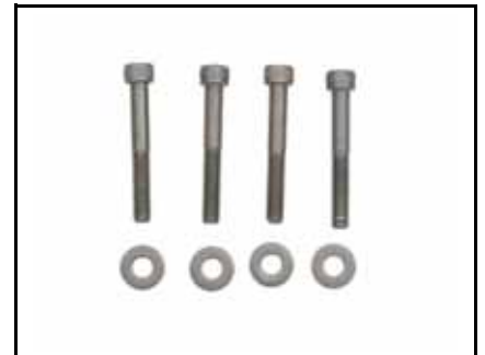
Flywheel removal, screw/washer kit 002581 P/N 5000007 (40/50, 60/70, 90-140) Use with 378103, Universal puller
