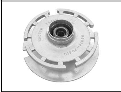
Test propellers (4-stroke): P/N 5032468 (25/30)(Use bushing, P/N 5034620 and stopper, P/N, 5034621) P/N 5032458 (40/50) P/N 5032478 (60/70) P/N 5034161 (90–140)
