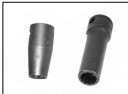
Torquing socket, rod screws 000797/50242 P/N 331638 (5/16 in. 12 point hex) P/N 346187 (3/8 in. 12 point hex)
