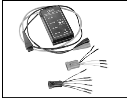
Ignition analyzer, 60°V carb models 23471 P/N 434017 – Includes 60° V6 harness kit, P/N 434127. Tests ignition sensor and allows static adjustment of idle and full advance ignition timing.
