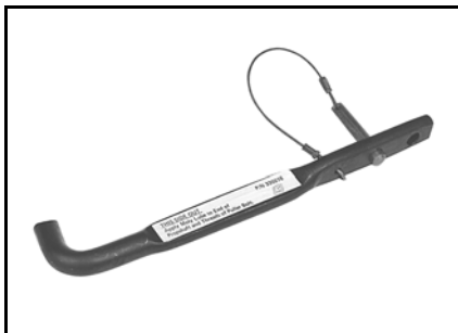
Puller, heavy duty (2 required) 2030 P/N 330278 (Use with body and screw from Universal Puller Kit, P/N 378103 to remove bearing housing)
