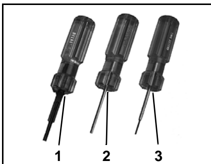
Amphenol connector tools: 1. Insert, P/N 322697 2. Pin removal, P/N 322698 3. Socket removal, P/N 322699 000798
