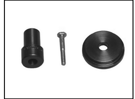
Installer kit, pinion bearing 002647 P/N 500009 Included in Driveshaft Shimming Kit (4-Stroke) P/N 5005926 (60/70)
