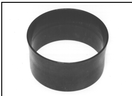
Ring compressors: CO3768 –Standard size P/N 336314 (60°V & 40–90 Evinrude E-TEC) P/N 326592 (40/50) P/N 326591 (25/30) P/N 339754 (9.9/15) P/N 326589 (6/8) –Oversize P/N 336313 (60°V & 40–90 Evinrude E-TEC) P/N 330222 (40/50) P/N 330223 (25/30) P/N 339755 (9.9/15)
