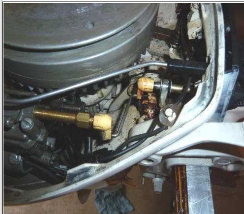
Here a view of the carburetor, showing synchronization screw head (red arrow) and flexible idle jet cable system
