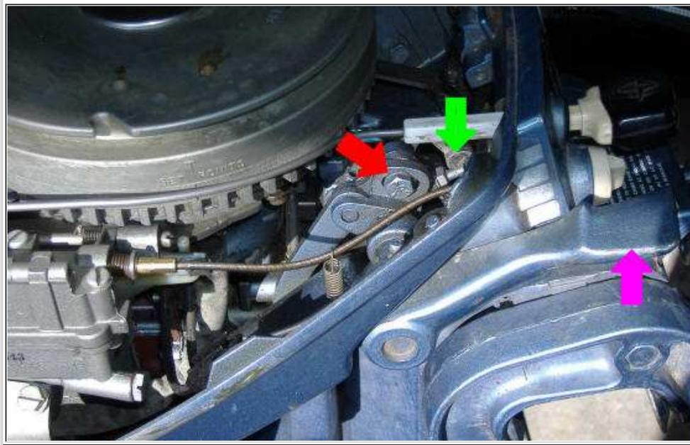
**Shift Gears :** On this model, the shift handle is on the outer starboard side (front RH looking forward). The positions are up for reverse and down for forward. The front panel of the motor has R/N/F printed vertically on the RH edge as seen in the photo LH below.
