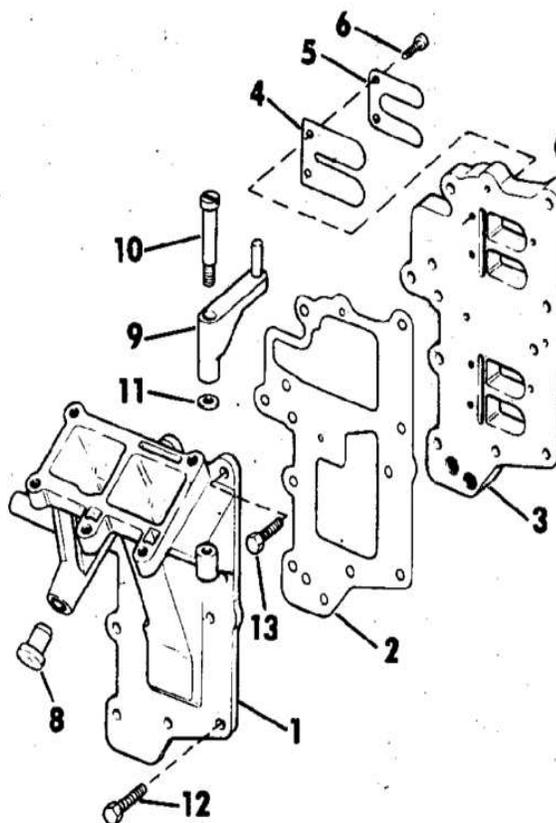
**Reed Valve Boxes :** As said above, the reed valves in these 9.5 motors were two different types. The early version used a set of reeds mounted in removable boxes that sat under the carburetor base and accessible only from that location. This adapter plate is held in place by two opposing Phillips head screws, which over time could become hard to remove without the aid of an impact driver as seen in the photo above. In this photo the reed box screws were already removed.
