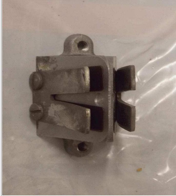
***Throttle Linkage :*** This linkage is rather different and complicated than you will generally see. The twist grip shaft has a small gear on the rear that engages a gear rack, so as you rotate the twist grip, this geared rack extends or withdraws. The rack shaft then engages a linkage plate that then engages another linkage plate, which ties to the timing plate. Rather complicated, but it works quite well.
