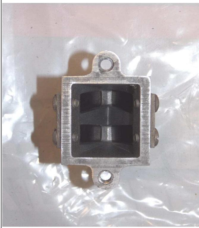
Here is the bottom view of the same reed box on the left, note the reed stops on the outside of the reeds
