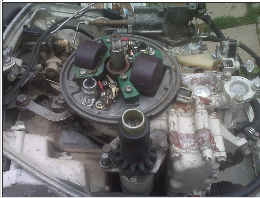
**Starter :** The manual recoil starter pull handle is located on the front lower part of the front panel. The actual starter is basically a manual copy of the automotive type starter system used extensively on may of the small OMC motors. There was no provision for a electric starter.
