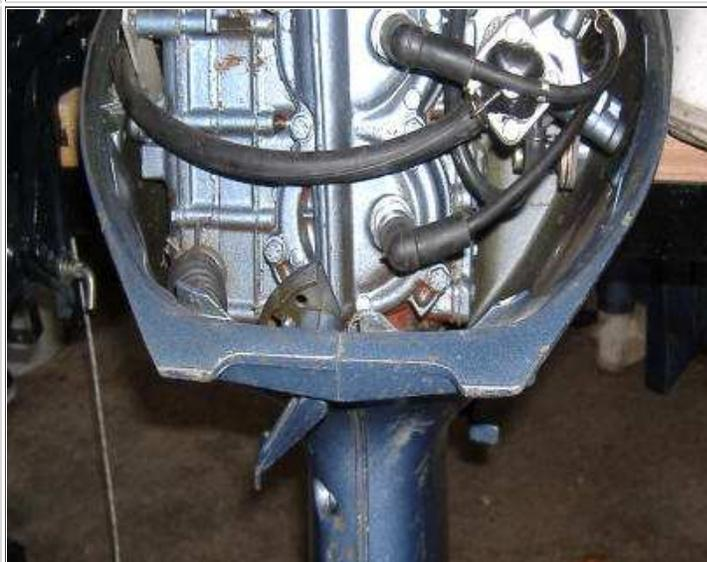
**Lower Cover :** These motors utilized a split lower cover that surrounded the exhaust housing. This feature compounds repairs where a simple part may need to be replaced, but the whole cover needs to be removed to access it.
