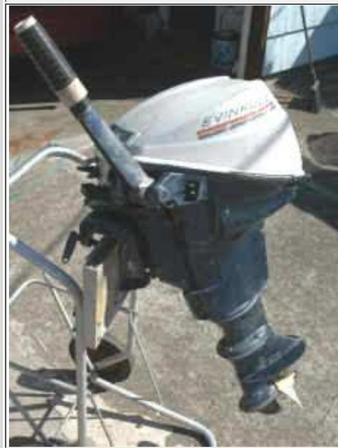
***Lower Units*** : The lower unit appears that they actually use the 4 bolt lower unit (gearcase) off the previous 10hp QD series.
