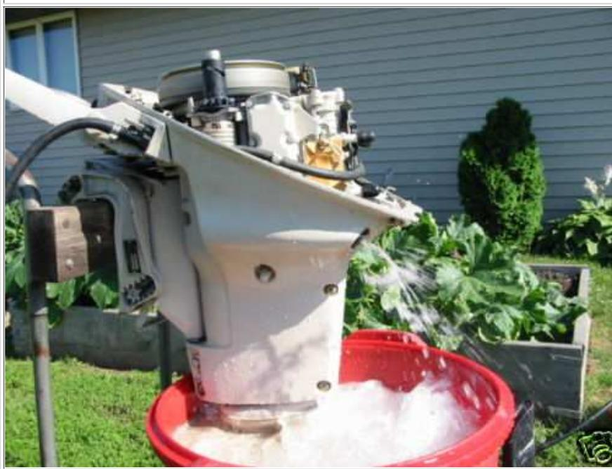
Water mix will only spray out that hole when the thermostat is open. So until the motor warms up, it should be dry for possibly the first minute or so when started cold. In the photo below, you will see the thermostat cover plate center top of the photo held in by the 3 bolts.
